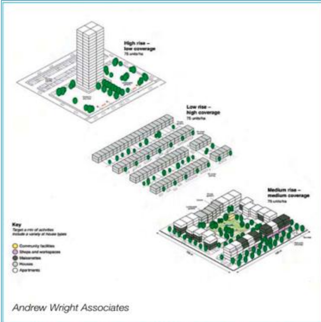
These three very different architectural forms are built to exactly the same density of 75 dwellings to the hectare.
